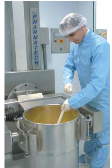
Sampling taken from a 200 litre Pharmatech drum
