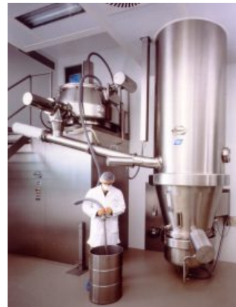
Installation showing a Diosna Mixer Granulator discharging in to a Diosna Fluid Bed Drier
