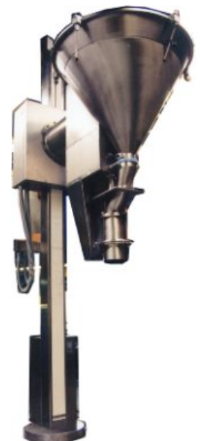
Fluid Bed Dryer Bowl Inverter with Mill. NB. unit connects to FBD bowl, lifts inverts and then mills the product
