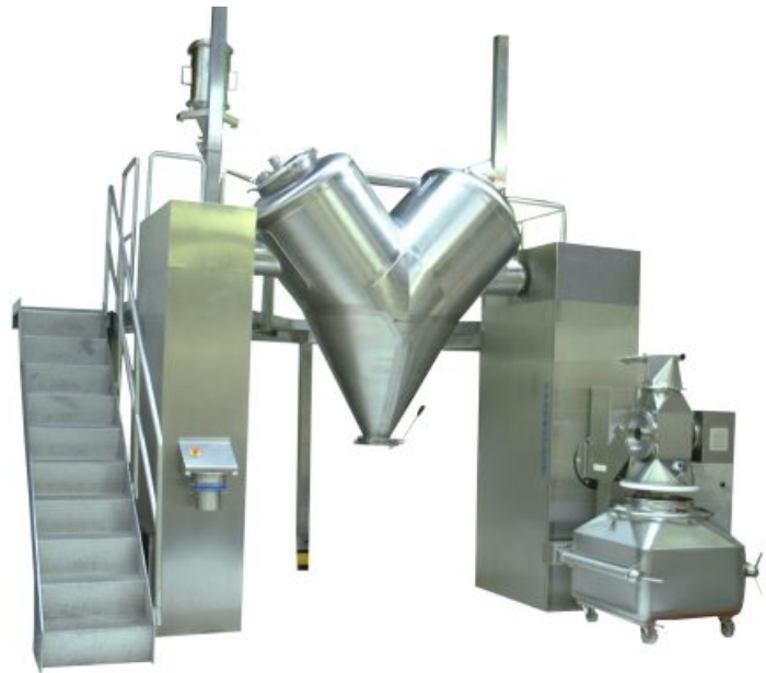
1500 litre V shell blender with operator gantry-loads by vacuum from Pharmatech IBCs
