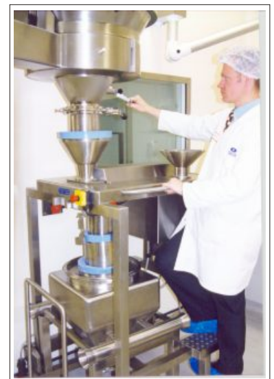
Dust Cap Seals being used to provide Dust free milling and charging of an IBC
